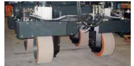
Larged sized load and drive wheels with rubber tires for diesel and gas powered transporters ensure high outdoor drive speeds, even on poor weather and ground conditions.
