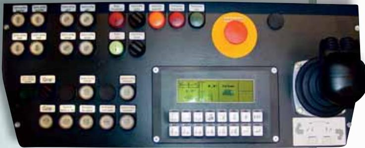
Clear arrangement and ergonomic placement of all operating elements and displays. Smooth operation of all hydraulic functions via joystick guarantees safe and careful glass handling. The standard electronic multidirectional steering system enables an exact truck positioning.
