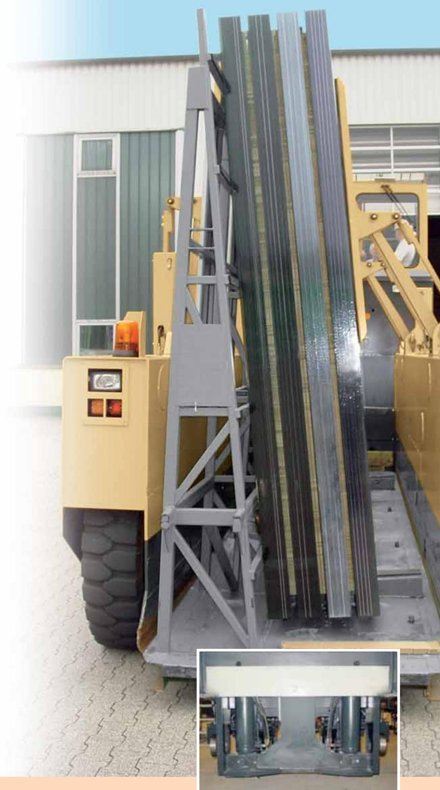
Horizontal standard glass clamps for minimum glass height 2.400 mm. Vertical glass clamps with increased retention force for thin glass and minimum glass heights of 1.600 mm (Option). Ultrasonic sensors installed on each clamp to avoid pressure on the glass pack.
