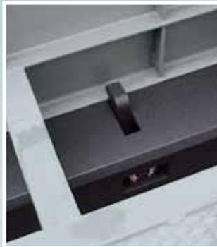
Special stillage securing system to stabilize unsymmetrically loaded stillages.
