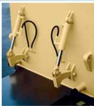
Special stillage securing system to fix an unsymmetrically loaded 30 tons A- and L-stillage.
