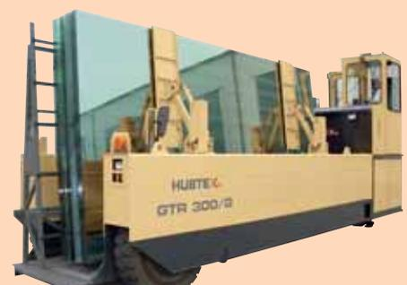
Driver's stand with bilateral, adjustable operator's panel for free visibility during truck manipulation with glass frame. Closed driver's seat cabin for combined indoor and outdoor application, optionally available with rotatable driver's seat, heating, and more.
