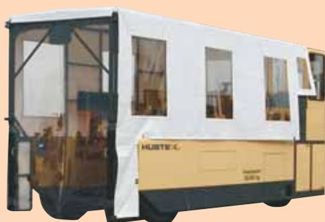
On request a pick-up type plastic cover as rain protection with wing doors to be opened and closed electrically from driver's cabin is obtainable.
