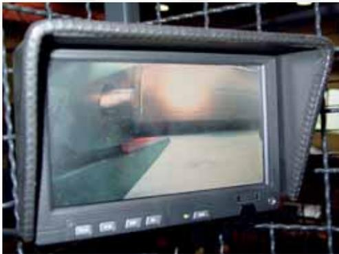
Two additional dashboards on each truck side for positioning of the side clamps and for improved view to driving direction.
