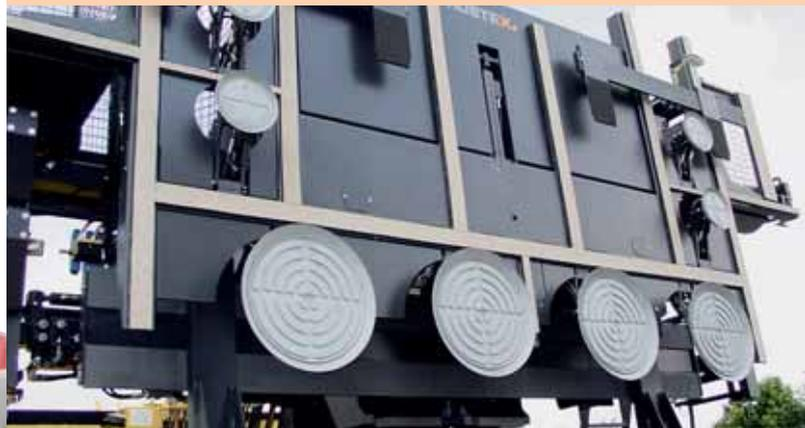
The suction cup rows of the integrated vacuum attachment for the handling of single glass sheets can be extended individually or combined. For the safe handling of broken glass the suction system is in addition individually or combined switchable.
