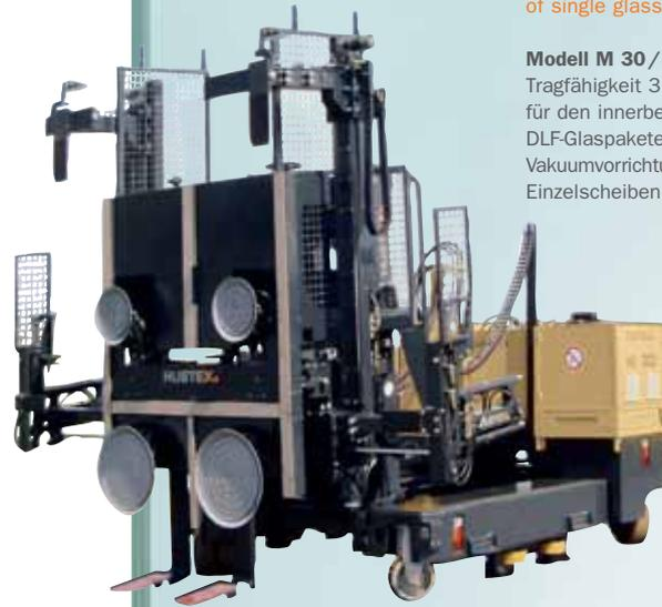
**Model M 30/ M 60 (1-man-version),** capacity 3.000 kg/6.000 kg for indoor transport of DLF-glass packs and vacuum attachment for the handling of single glass sheets.
