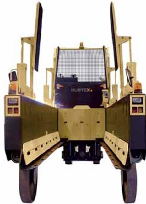
**Electric Glass Frame Transporter, model GTR 330/E, capacity 33.000 kg**
