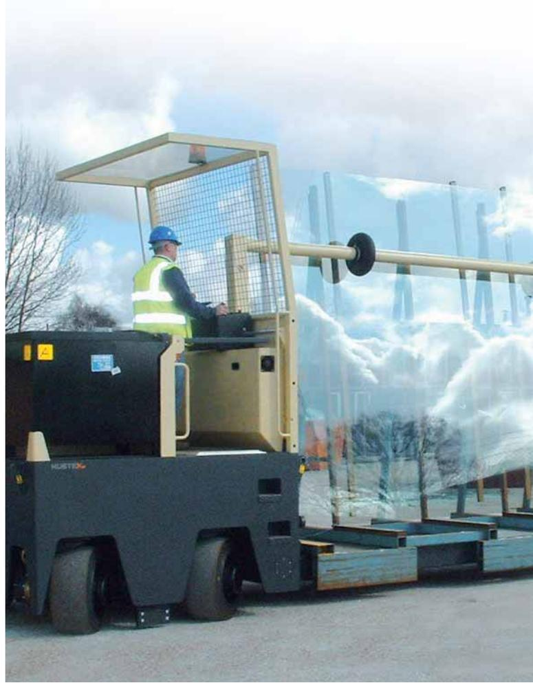
As a third solution for indoor transport of A- and L-stillages with feet HUBTEX offers a complete range of platform trucks, GTT-series, with capacities up to 33 tons. Stillage take-up by driving under the stillage and lifting of platform. The truck "highlight" is a compact design with an extremely small turning radius.
